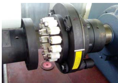
Torque limiter-the overload protection torque limiter
